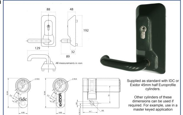
This OAD is manufactured from stainless steel which helps prevent force and drill attack, and incorporates cylinder protection to prevent manipulation. When locked, the mechanism is disengaged allowing the lever to move freely. When unlocked, the lever, spindle, and mechanism engage allowing the bolts to be withdrawn from the outside. The lever remains engaged until it is re-locked.
